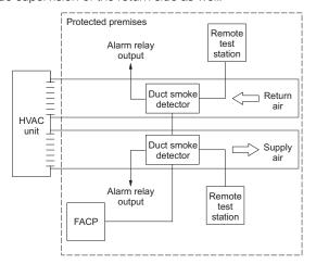
SuperDuct detectors continually sample air flow in the HVAC duct and initiate an alarm condition whenever smoke is detected. An alarm is activated when the quantity (percent obscuration) of combustion products in that air sample exceeds the detector's sensitivity setting.
