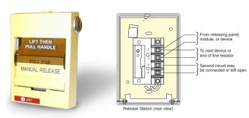
The manual release station is a normally-open, dry contact signal initiating device. The 276A-REL is a single-action station that requires the user to pull the release handle to initiate the release of a fire suppression agent. The 278A-REL (shown) is a double-action station that requires the user to raise the upper door, then pull the release handle to initiate the release.
